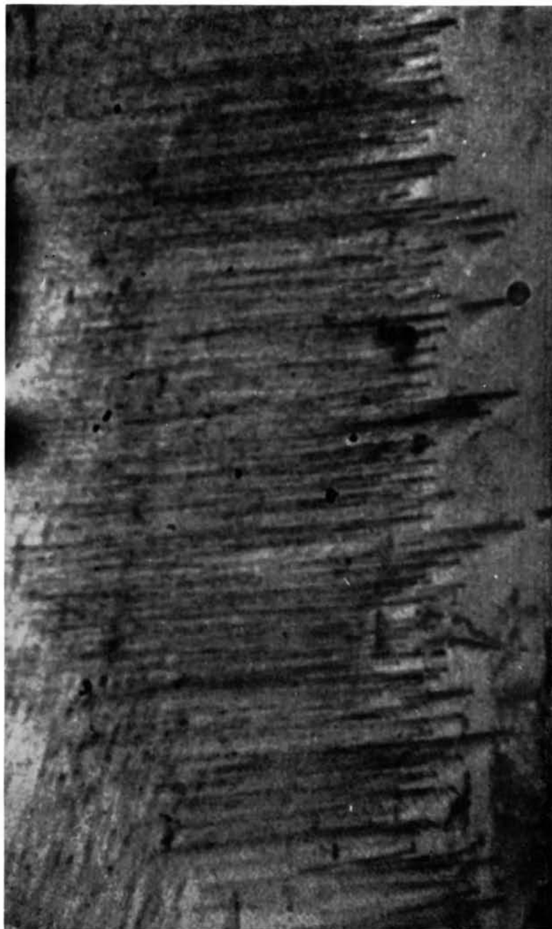
Fig. 2. X-ray topograph of an oxalic acid dihydrate single crystal showing groups of straight dislocations arranged in sheet-like arrays. Cu K\alpha_1 radiation ( \times 100 ).
